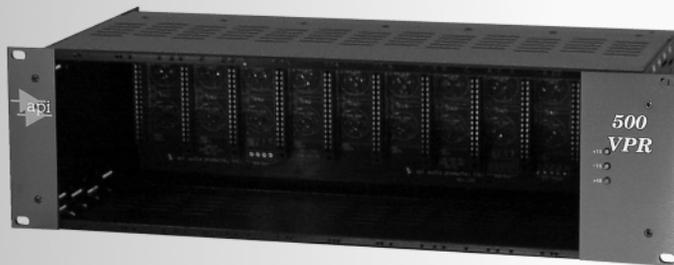
The API Model 500V is powered externally by a tri-polar power supply and is designed to accept many different API standard format 5.25" x 1.5" modules. The 500V comes internally wired for PIN 2 hot. Any external dual 16 volt power supply can be used, or the API 200PS can be purchased. The input/output jacks are both XLRs. The 500V can hold up to ten API modules, regardless of the "era".
